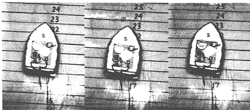
Figure 13. Robotic swimmer with muscle undulation frequency of 3 Hz (frame time interval, 1/3 second)
